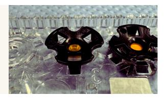
The three prongs of the clip should snap into three of the six openings around the central window. Ensure that you feel a secure snap from each prong latching onto the opposite surface so that the windows is held tightly. In rare cases, one or more of the prongs may be defective and not hold tightly – in that case, please toss the clip and use a new one.
