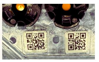
Don't forget to carefully record the assignment of QR codes to specific samples. You can easily double check the string associated with the QR code using any common QR reader, such as with most general phone camera apps, or e.g. Google Lens.
