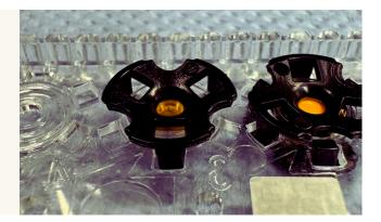
The three prongs of the clip should snap into three of the six openings around the central window. Ensure that you feel a secure snap from each prong latching onto the opposite surface so that the windows is held tightly. In rare cases, one or more of the prongs may be defective and not hold tightly – in that case, please toss the clip and use a new one.
