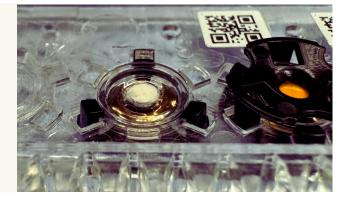
That being said, avoid over-filling the slot. The polyimide windows should still lay flat against the powder and holder. Otherwise, the contribution of the background intensities will be slightly modified.
