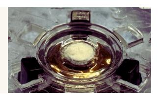
If a lot of powder does spill outside of the well, you can use a cotton swab wetted with some solvent to clean the excess around the edges or other surfaces of the sample holder.
