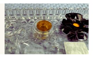
Ensure that the window is centered over the opening for best surface contact.
