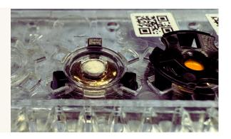
That being said, avoid over-filling the slot. The polyimide windows should still lay flat against the powder and holder. Otherwise, the contribution of the background intensities will be slightly modified.
