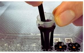
For best quality measurements, the powder should fill the window completely and densely. This ensures both that the maximum sample cross section is available for best possible data statistics, and maximizes the orientation distribution of the crystallites for acquisition of complete Debye–Scherrer rings.
