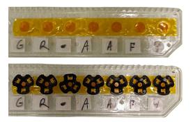
Loaded sample holders are kept under **argon** until just before measurement.
