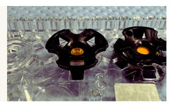
The three prongs of the clip snap into three of the six openings around the central window holding the window tightly in place. Though tightly fitted, it is not perfectly sealed against ambient air. For air sensitive materials, preparations can be performed in a glove box and stored under inert gas until the measurements are performed.
