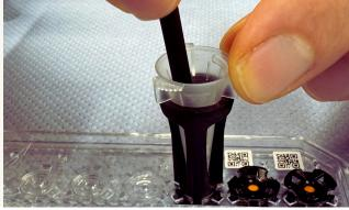
For best quality measurements, the powder is filled completely and densely into the well. This ensures that the maximum sample cross section is available for best possible data statistics, and it maximizes the orientation distribution of the crystallites for acquisition of complete Debye–Scherrer rings. During measurements, we additionally shake the sample holder and scan the beam across the window to further improve the sampled volume.
